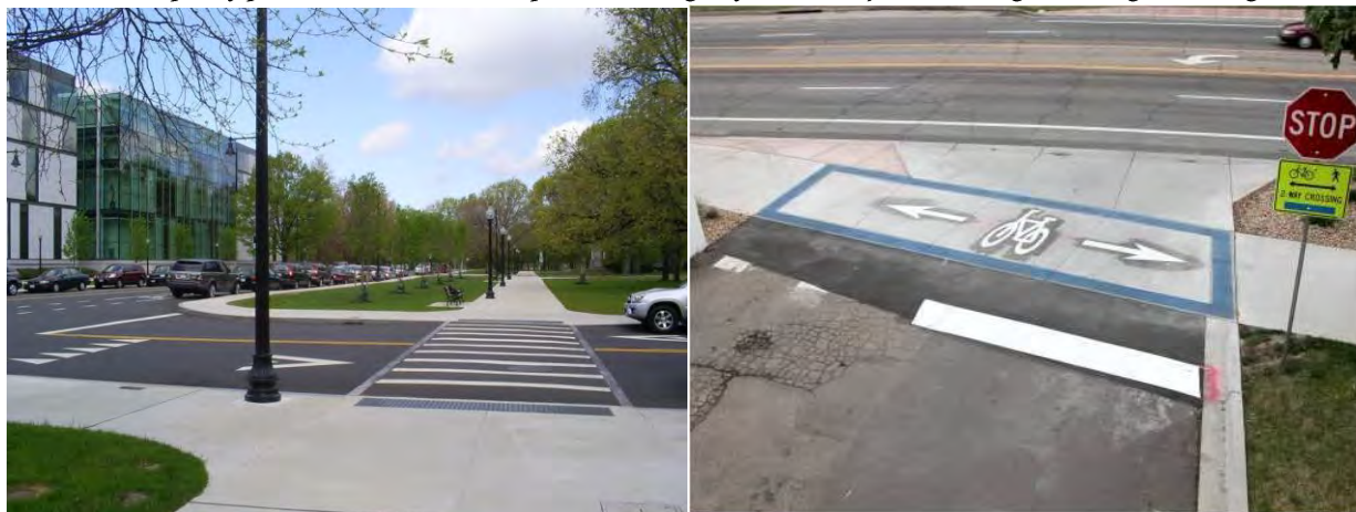
Example of prominent shared use path crossing (left) and bicycle crossing marking used (right)
